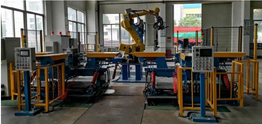
Intelligent Casting Production Line (The robot is used to realize automatic casting for clamps.)
